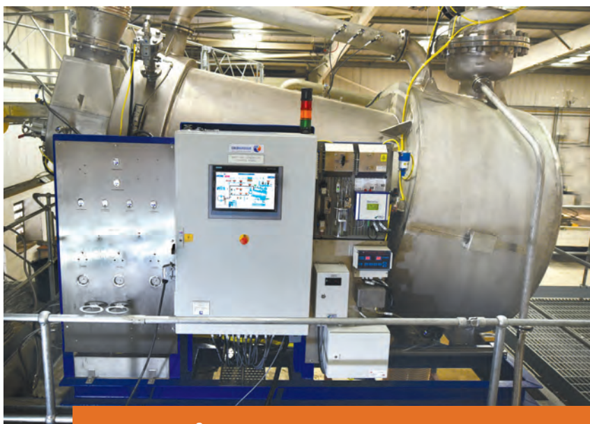
4000Nm³/hr Sea Guardian™ Inert Gas Generator on test at the Coldharbour UK test facility
